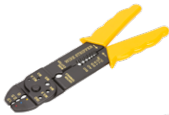
KH-502 8" Crimping tool for insulated terminals 0,5 - 6,0 mm 2 Bolt cutting M2,6 / M3 / M3,5 / M4 / M5 Wire stripping 0,75 - 6,0 mm 2
