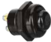
AE-ZZ107 Push button switch On-Off 20A@12V 2 Screw contacts Installation dimension Ø 22,5 mm
