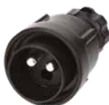
2 Pole waterproof break-proof metal plug Silver plated crimp/solder contacts With rubberized metal screw ring IP54, IPX4, IPX7 protection
