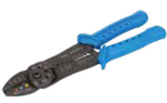
MEB-700C 9" Multi-tool for insulated ( brazed seam only ) and open barrel terminals 0,5 - 6,0 mm 2 Bolt cutting M2,6 / M3 / M3,5 / M4 / M5 Wire stripping 0,75 - 6,0 mm 2
