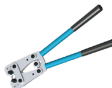
KHB-50 15,3" Crimping tool for non-insulated terminals 6,0 - 50,0 mm 2 HEXAGONAL crimp
