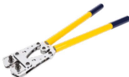
KHB-120 26" Crimping tool for non-insulated open barrel flag terminals 6,0 - 120,0 mm 2 HEXAGONAL crimp
