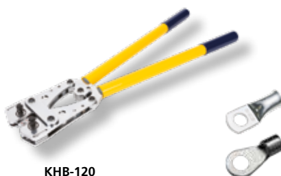
KHB-120 26" Crimping tool for non-insulated terminals 6,0 - 120,0 mm 2 HEXAGONAL crimp
