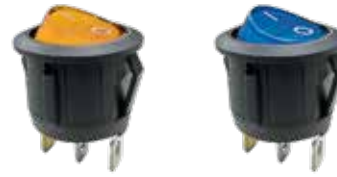
AE-ZZ225 Rocker switch On-Off-On 16A@12V 3 Tab contacts 4,8 x 0.8 mm Installation dimension 19 x 13 mm
