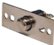
AE-ZZ011 Door contact switch On-(Off) 5A@12V 2 Screw contacts Installation dimension Ø 18,5 mm
