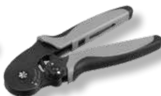
92146 8,3" Crimping tool for cord end terminals Twin wire 2x0,5 - 2x10,0 mm 2 HEXAGONAL crimp
