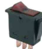
AE-ZZ233 Rocker switch with red LED On-Off 20A@12V 3 Tab contacts 6.3 x 0.8 mm Installation dimension 30 x 12 mm
