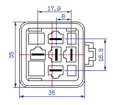
DIMENSIONSL x W:35 x 35 mmTECHNICAL SPECIFICATIONSApplication:For RE620Q series (40A, 5 pins) auto-<br/>motive relays<br/>Special feature:<br/>Wire length:Source and a series (40A, 5 pins) auto-<br/>motive relays<br/>Waterproof<br/>200 mm
