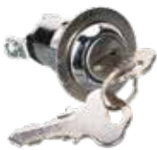
AE-ZZ145 Burglar alarm switch with 2 keys With dust shutter Off-On, 12V 2 Screw contacts Installation dimension Ø 21,5 mm
