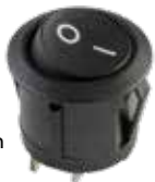
AE-ZZ223 Rocker switch On-Off 16A@12V 2 Tab contacts 4,8 x 0.8 mm Installation dimension 19 x 13 mm
