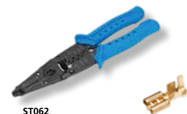
ST062 8,5" Multi-tool for crimping Non-insulated ( brazed seam only ) terminals 0,5 - 2,5 mm 2 Open barrel terminals 0,25 - 1,5 mm 2 Coaxial cable connectors 6,0 mm Wire stripping 0,25 - 4,0 mm 2
