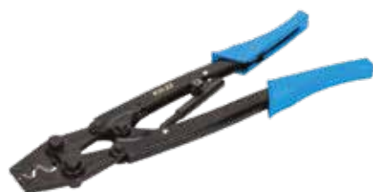
KH-22 14,4" Crimping tool for non-insulated terminals 6,0 - 25,0 mm 2
